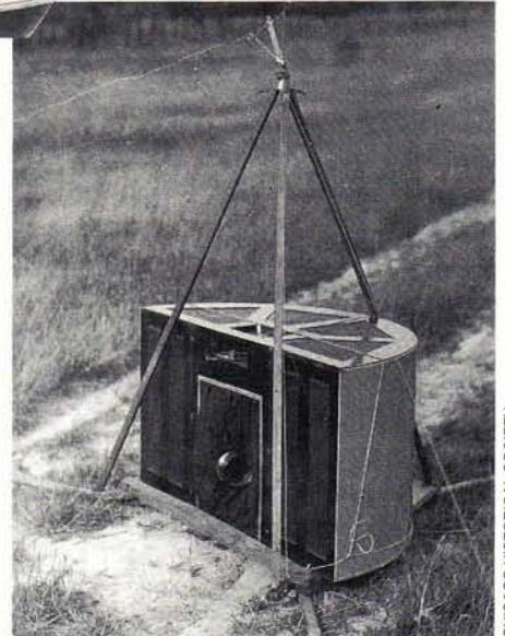
the flattened-cone focal plane shutter. In order to reduce the comparatively abundant sky light and allow for a longer exposure of the darker land surface, he varied the width of the slit. The image reached the film upside down so he made the slit wider on top to increase the length of exposure of the darker land surface.
