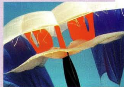
CLOSE-UP: a view into the "jet port" at the trailing edge of a Flow Form shows how panels separating cells have large, circular vents, which help create pockets of pressure. (The strings were sewn in to simulate air flow.)
