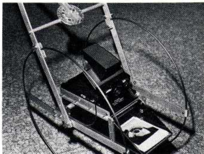
Below, Curtis Marshall's rig for kite-lofted photography using a Polaroid SX-70.
