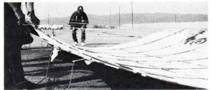
Left, the end line from each row of six is matched with the other five. To assure that each row is exactly centered, end lines are matched to each other by being crossed over to opposite side and brought out front. When they are matched, close to the kite, the marker-man holds tightly as all six lines are stretched evenly to him. Each row is measured and tied in a loose slip knot. Top center, to impart a bow and dihedral to the kite, the center lines in each row of six are shortened. Here, Taro Suda uses the "finger-measure" method (others use a ruler). Bottom center, each row-bundle is matched at the mark on one (end) line and the whole mass bound and formed into a rope. Top right, the kite is now turned over, face down (notice the flexibility). Bottom right, bow lines help the bridle to shape the kite's dihedral. Bowing is deeper at the trailing edge, but the second-to-last bow is a bit more bowed than the last rib (bone). Each kite requires its own bridling and expected winds on the day of flight are also taken into consideration. ◇
