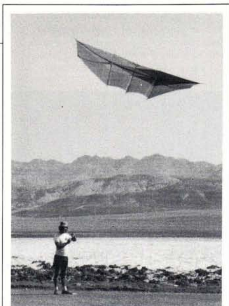
Nop's kite, the Genki (meaning health in Japanese) was originally double-spined. Nop added the third spine to the kite (down the center) for use in trains and aerial photography. The aspect ratio may vary between 1.5 to 1 and 4 to 1. The measurements given here (in centimeters) are a good average.
