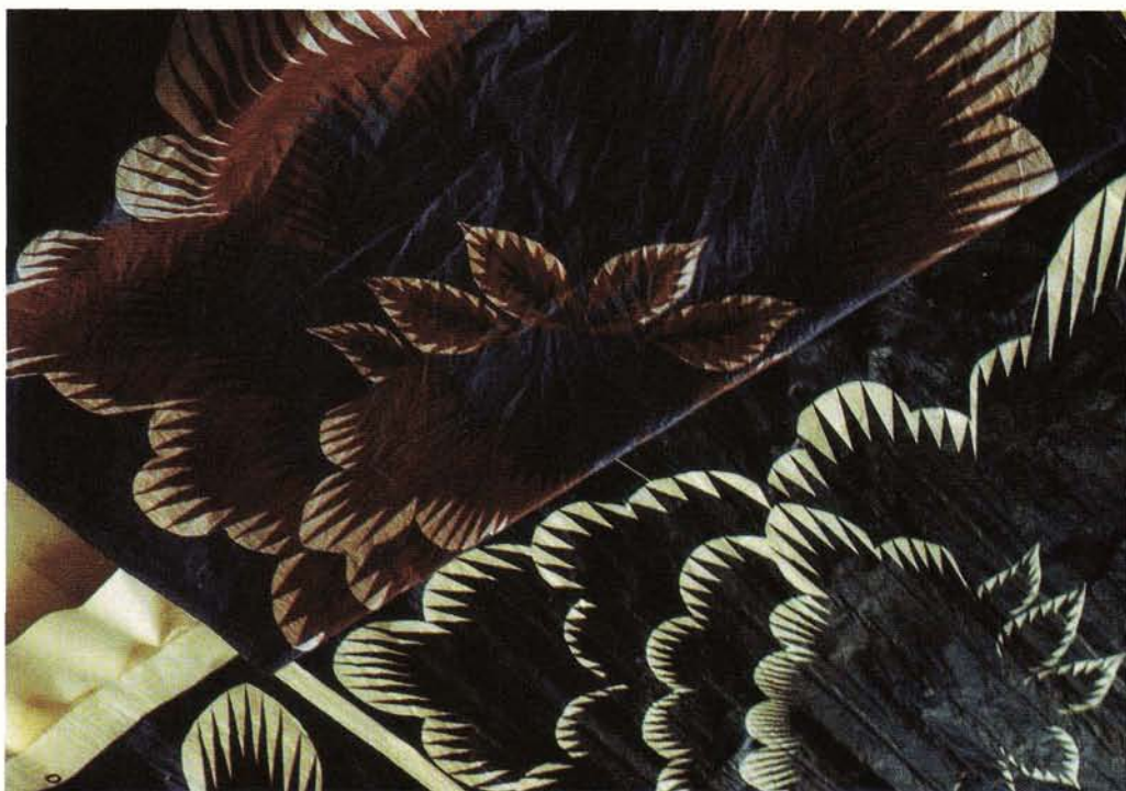
Opposite: dye mixing bench. Above: comparison of lotus print unsteamed (dark) and steamed (bright).
