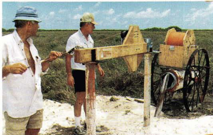
A winch beam mounting is quickly made of island scrap. It works!
