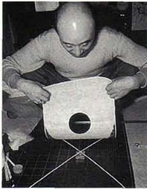
Right, Mr. Woo shows his device for preparing cutting line. The line is pulled from the first cylinder down inside a can containing epoxy resin (plus hardener) and artificial diamond powder. The line then runs through a cotton cloth to clean off excess resin, then through a simple guiding mechanism to ensure a very regular winding onto a second cylinder, where it dries. With this device, Mr. Woo can make 24,400 feet of cutting line a day.
