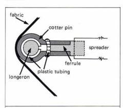
cotter pin . . 0.125" diameter x 2" long ferrule . . . . 0.248" outside diameter spreader . . . . . 0.250" inside diameter box kite . . . . . . . . 108" x 32" x 32"
