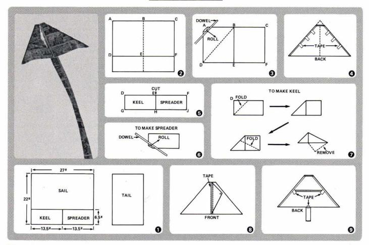
The Comics Kite is a kite without spars, that is: without spars in the traditional sense (wood, plastic, fiberglass, etc.). Instead, the spars—plus sail, keel and tail—are made from sheets of newspaper.
