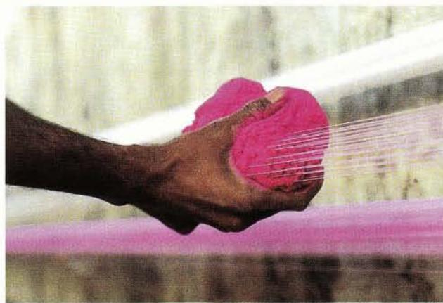
**Manjha by the mile:** glass-coated flying line is prepared in any available space, including, as above, the streets. Left and lower left, the preferred technique is to apply the thick mawa or *luggdi* by hand. Lower right, another, faster method involves dipping the "threads" in a liquid mixture and rolling them on wheels for drying, but the line is lessened in strength and cutting ability.
